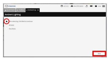
9. Check the vehicle ignition status is on, and click "Next" button. (Do not engine run)
